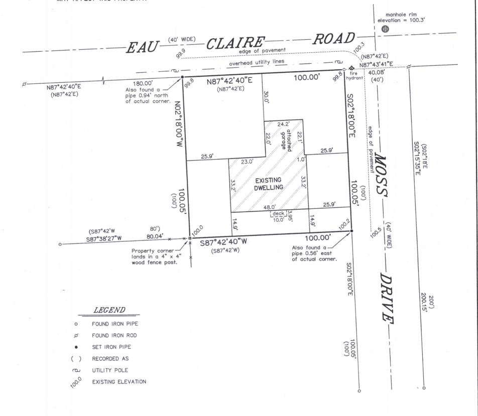
BEARINGS HEREON RELATE TO THE EAST LINE OF BLOCK 97 OF PELL LAKE SUBDIVISION SECTION 3. ASSUMED BEARING OF SOUTH 02°18'00" EAST AS PLATTED.
